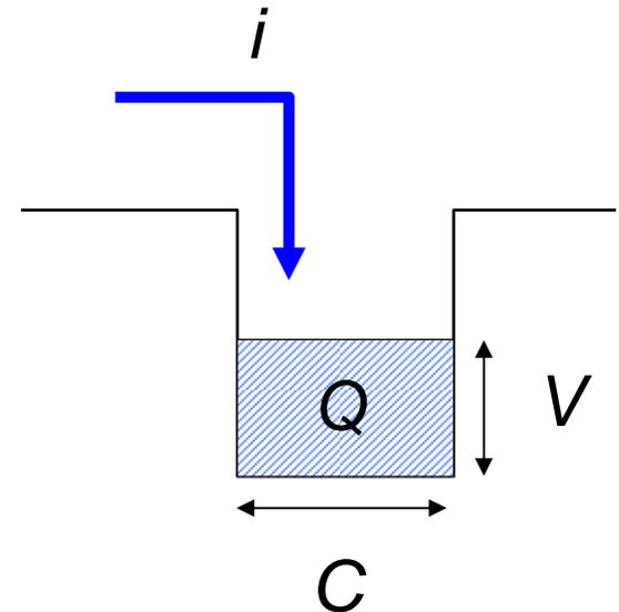
Photocurrent is *integrated* over a certain integration time in a pixel *while the other pixels are read out*
