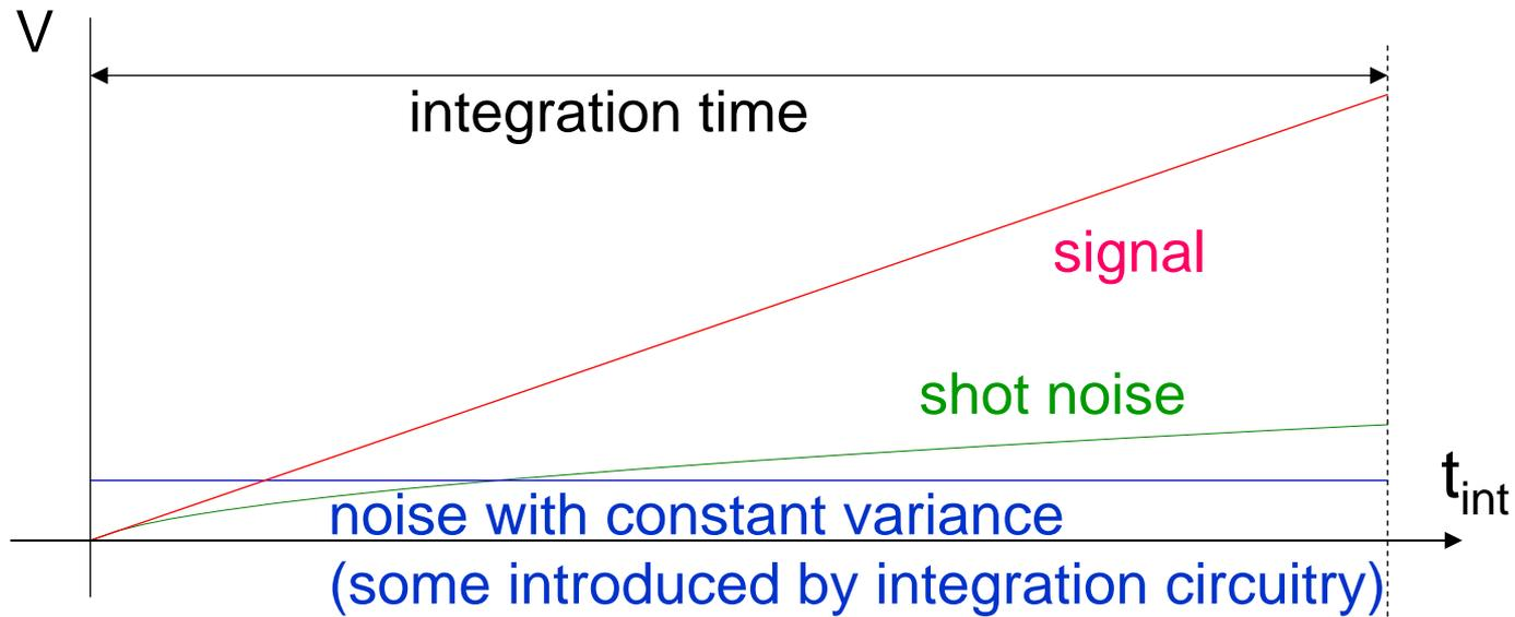
$$V_{\text{signal}} = \frac{i_{\text{signal}} t_{\text{int}}}{C} \quad V_{\text{shot,rms}} = \frac{Q_{\text{shot,rms}}}{C} = \frac{\sqrt{e \bar{i} t_{\text{int}}}}{C}$$
