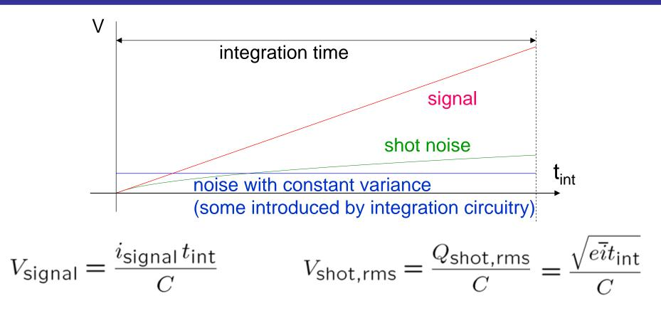
With N times longer t<sub>int</sub>, signal-to-noise ratio (SNR) is multiplied by:
