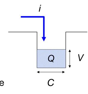
C: capacitance of the node where the charges are integrated
