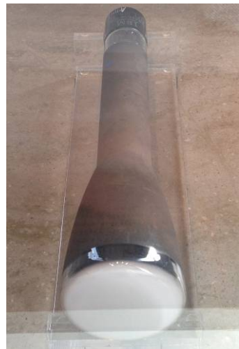
陰極線管 (Williams-Kilburn管)
