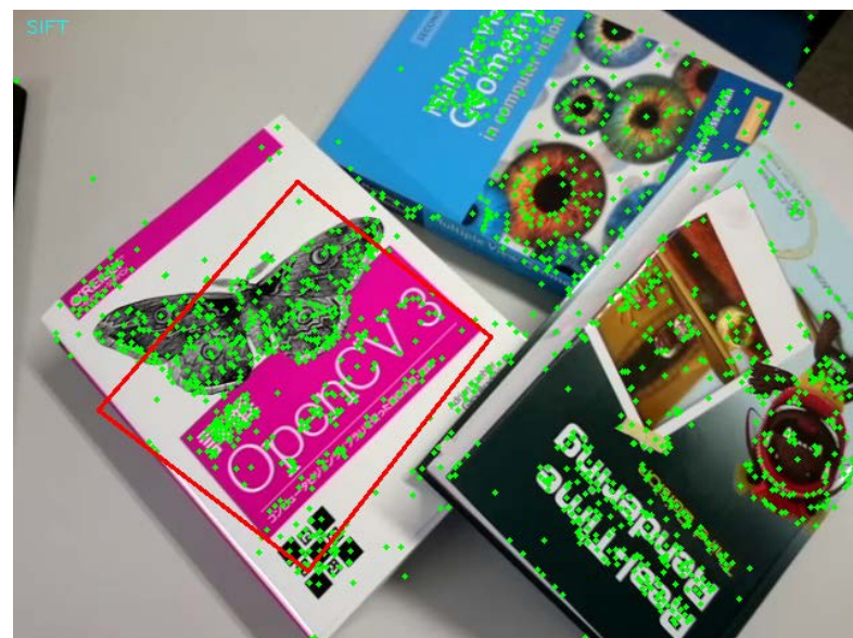
Estimation of homography transformation using the matched keypoint pairs
