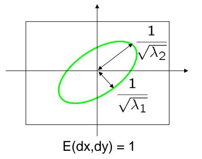
$$E(dx, dy) = (dx, dy)H\begin{pmatrix}dx\\dy\end{pmatrix} = 1$$
