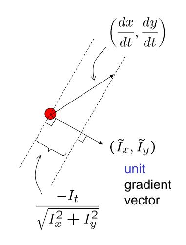
Thus we cannot determine the optical flow from  $I_x$ ,  $I_y$  and  $I_t$ . Additional assumptions are needed.
